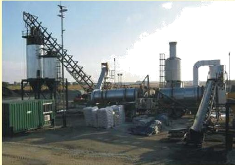
Figure 2. Mobile asphalt mixing plant capable of handling at least 40% RA
